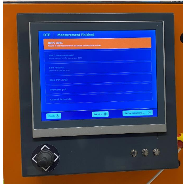
Figure 2. An alarm from the device to repeat sampling due to suspicious measurements.
