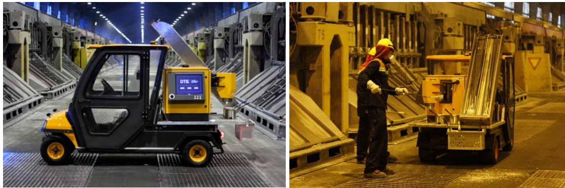
Figure 1. Portable elemental analyzer mounted on an electric vehicle (left). A liquid metal sample is extracted and poured into a ladle clamped to the analyzer platform (right).
